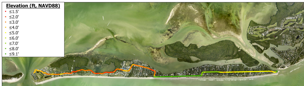
Figure 37. Captiva Evacuation Route Elevation
