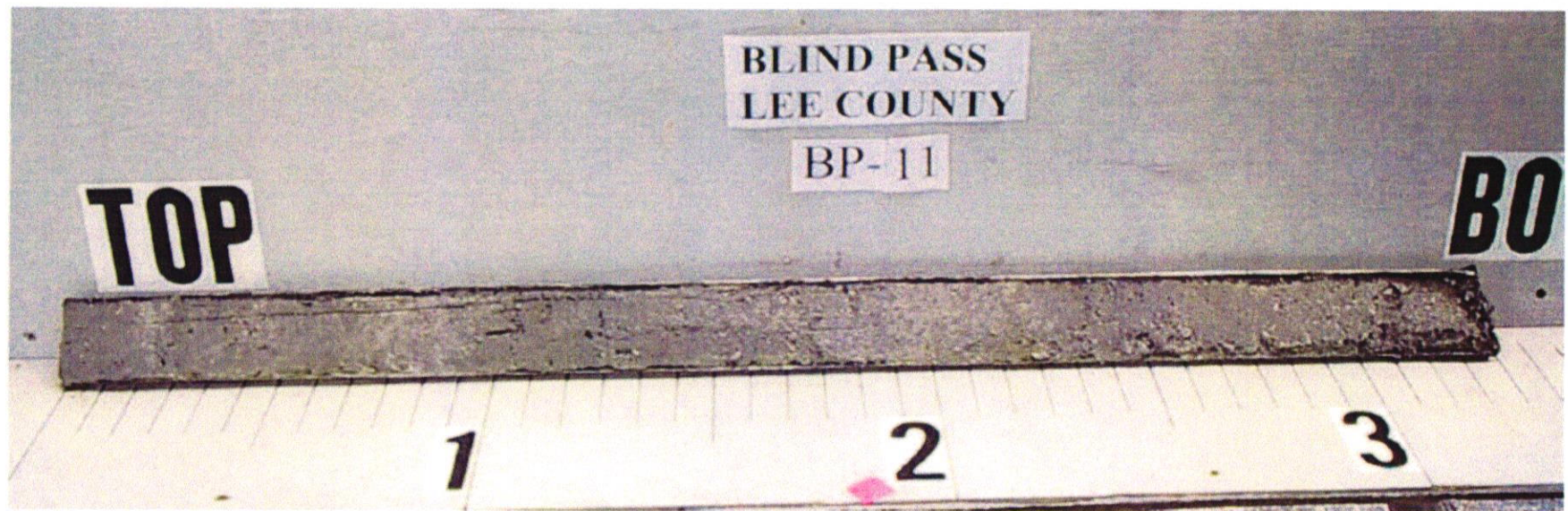
Photo 14 Vibracore BP- 11 (Bottom) -7.2 to -10.6 NAVD
