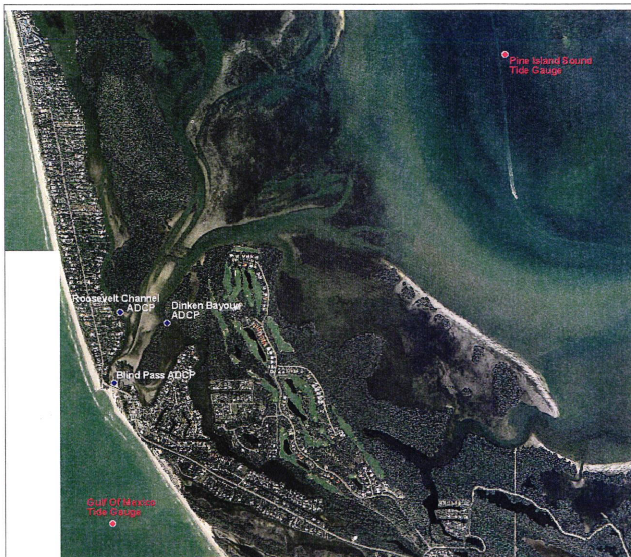
FIGURE 10 LOCATION MAP OF TIDE GAUGES AND CURRENT PROFILERS (ADCP)
